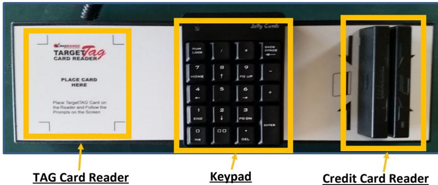
Step 1: Place your countdown card (TAG Target card) on the TAG Card Reader. The screen will automatically advance to the “Add Targets” screen.
